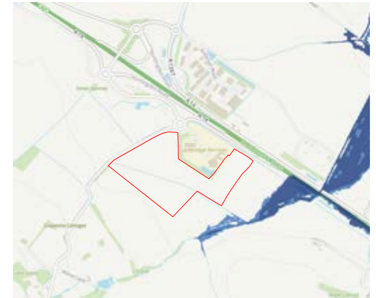
Figure 22: Site's location on the EA Flood Risk Map - Rivers and Seas (EA Flood Map)
