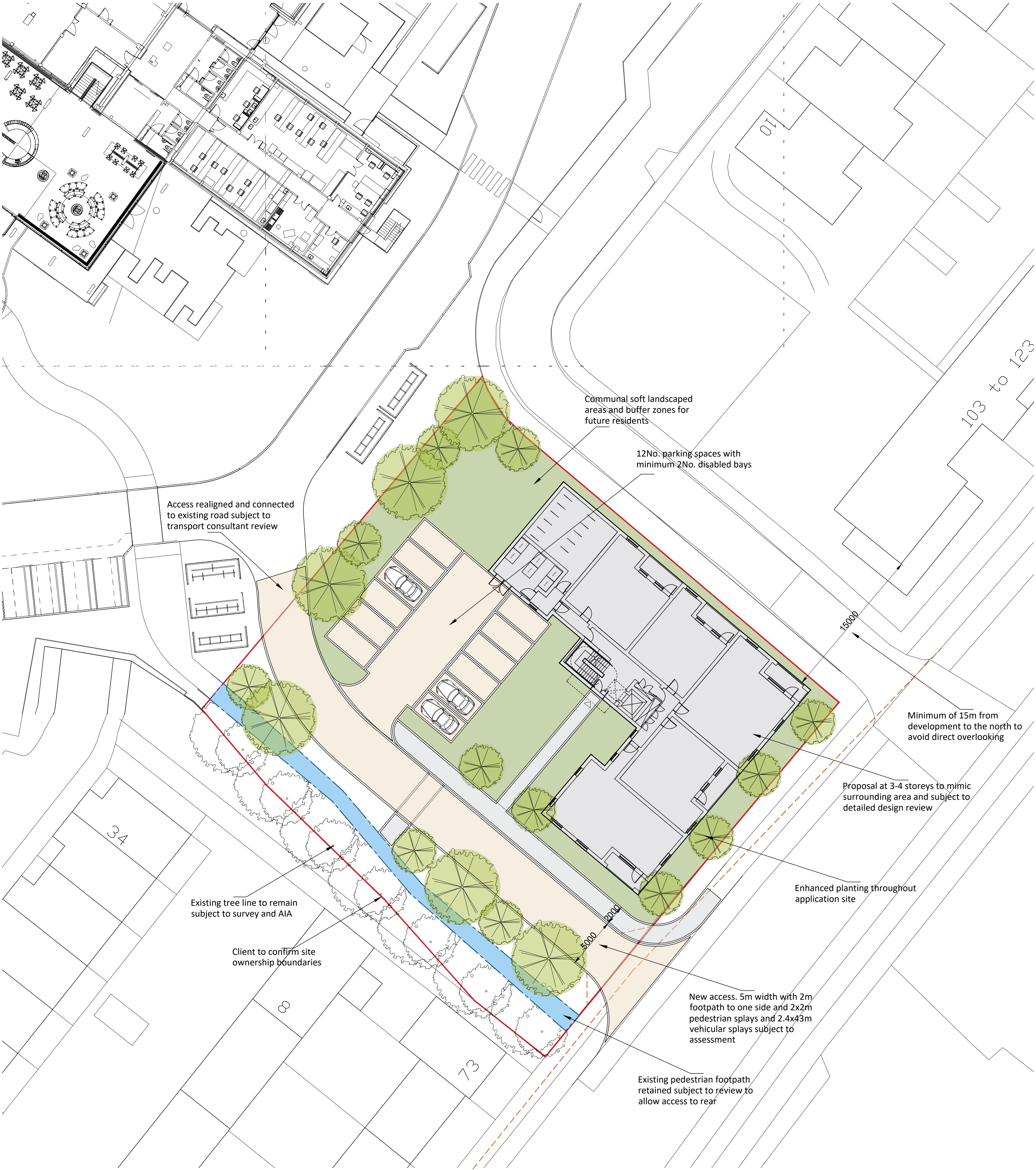
PROPOSED GROUND FLOOR PLAN 3No. 1 Bed Apartments 2No. 2 Bed Apartments
