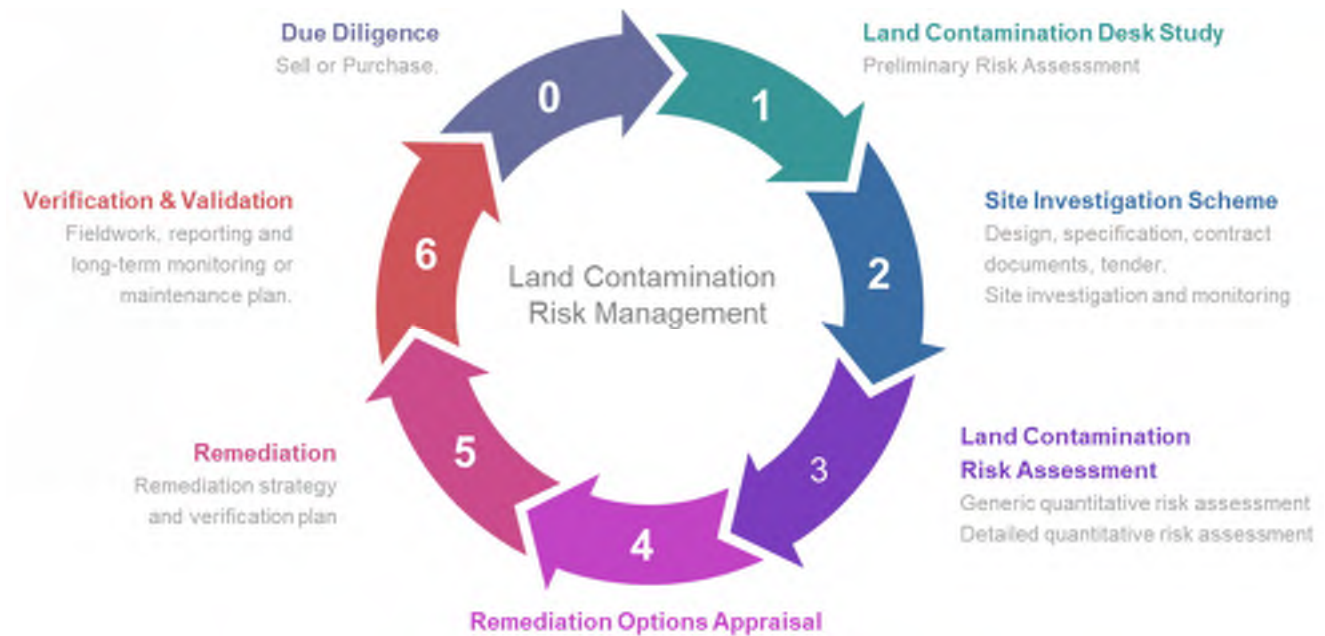
Figure 13 Land Contamination Risk Management process - simplified
