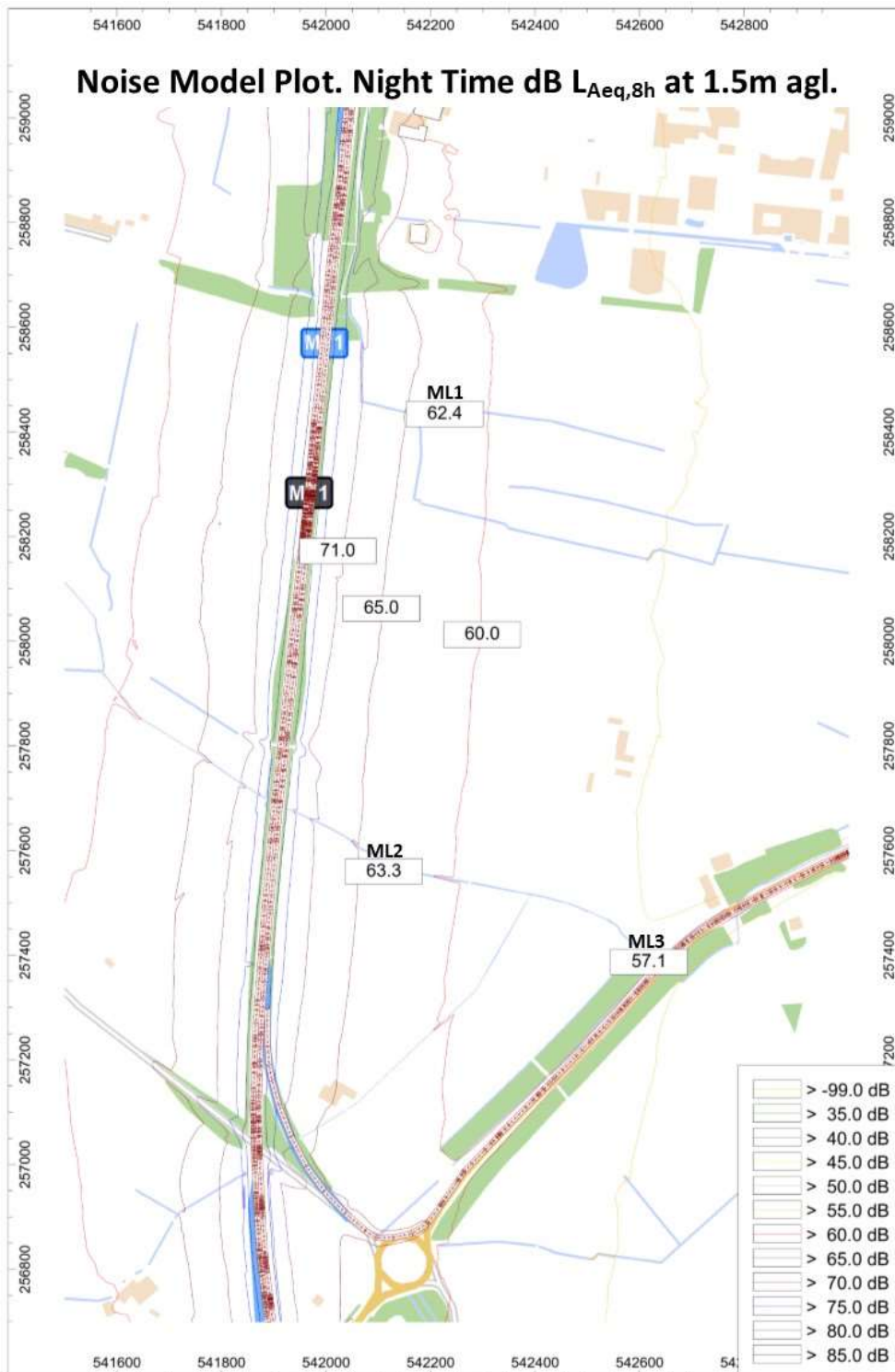
Figure 7 – Initial Night Time Noise Model Plot, Grid Spacing 2m, Grid Height 1.5m, dB L Aeq,8h
