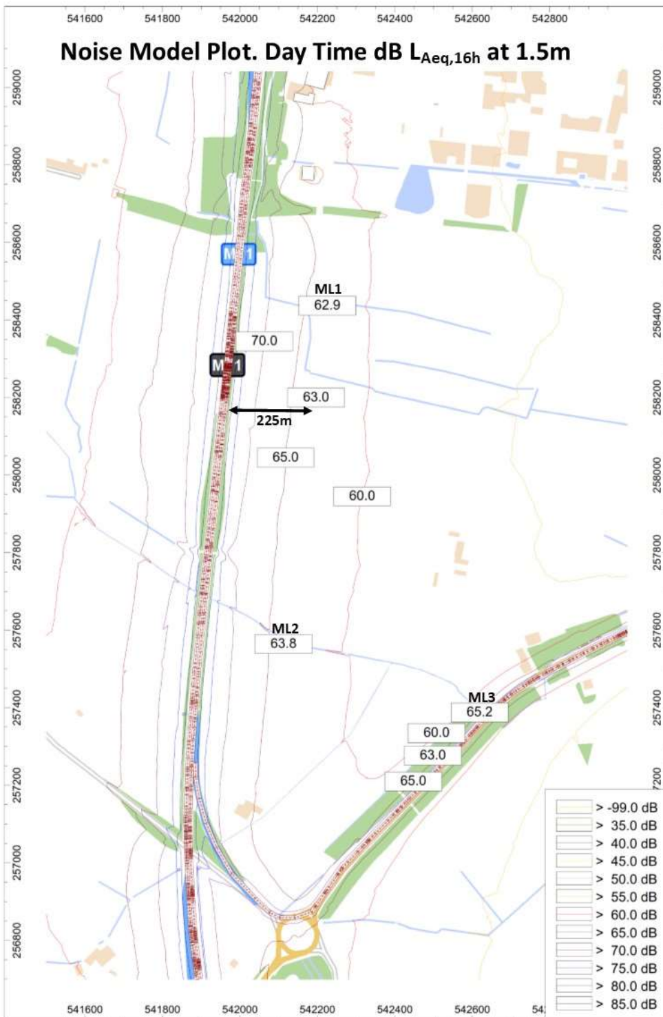
Figure 6 – Initial Day Time Noise Model Plot, Grid Spacing 2m, Grid Height 1.5m, dB L Aeq,16h
