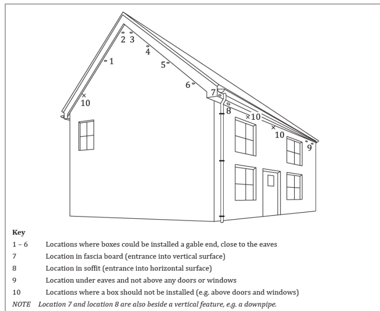
Figure 6: Suitable locations for the installation of nest boxes in a typical residential home (from BS 42021:2022)
