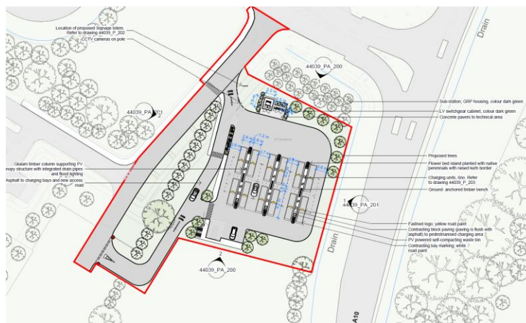
Figure 2: Approved EV charging facility site plan
