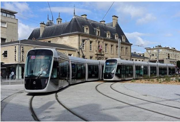
**Figure 18.** Caen: population ~107K. Light rail replaced bus rapid transit because rubber tyred vehicles rapidly wore out roads (tracking), leading to high operational maintenance / costs, and impacting reliability / ride quality / patronage.
