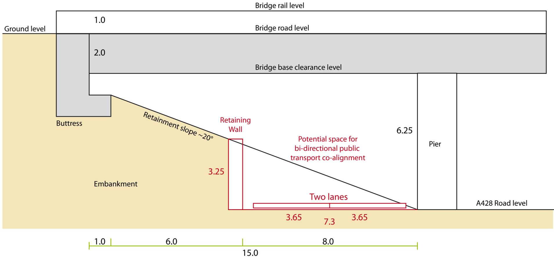
Madingley dimensions - 15.0 m from pier to buttress edge, 6.25 m height from A428 road level to clearance under bridge.
