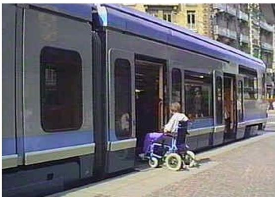
Figure 15. Accessible light rail vehicle in Grenoble.
