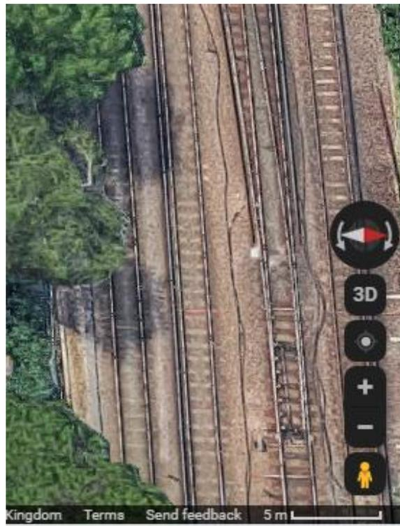
**Figure 4:** Croydon Tramlink alignment immediately west of Beckenham Junction station. The light rail line is at far left, while the remaining three lines are heavy rail. (Image: Google Maps 2019).
