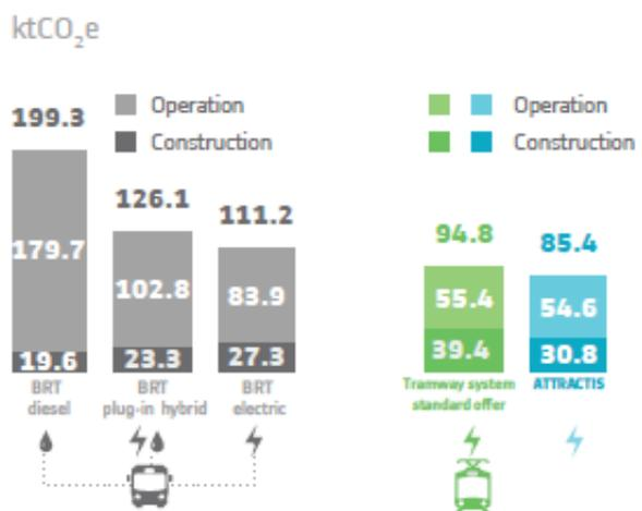
Figure 13. Carbon footprint of Bus Rapid Transit vs light rail.
