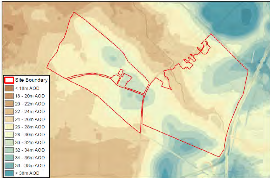
Figure 2.2: LiDAR Area Topography of the site
